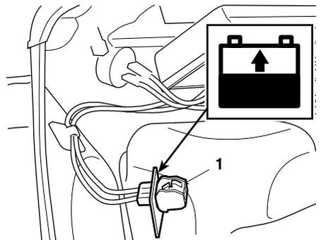
The machine comes with a connector (1) for recharging, to be connected to the cor-
