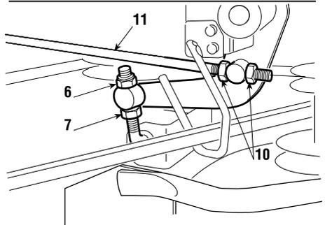
If the front part rises too early or too late, you can regulate the movement by turning the nuts (10) on the connecting rod (11).
