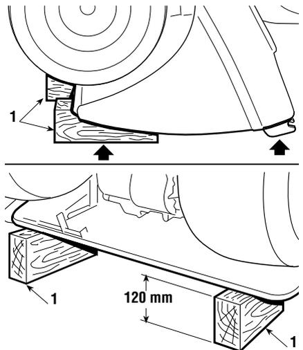
**⚠ DANGER!** Check that the machine is stable before doing any work
