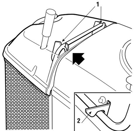
If you would like to mow without using the grass-catcher, an optional stone-guard kit (☛ 8.2) is available. This has to be attached to the rear plate as indicated in the relevant instructions.
