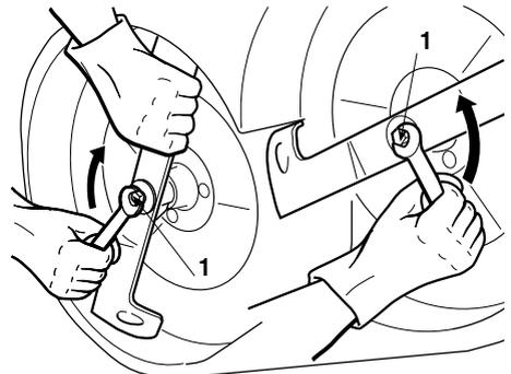
Sharpen the two cutting edges using a medium grade grinding wheel and check the balance by holding the blade up with a round 18 mm Ø bar inserted in the central hole.
