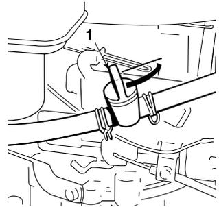
When the engine has started, put the accelerator in the «SLOW» position.
