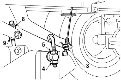
Any difference in height from the ground between the right and left side of the deck can be compensated by turning the two nuts (4 – 8) and locknuts (5 – 9) of just the back rods.
