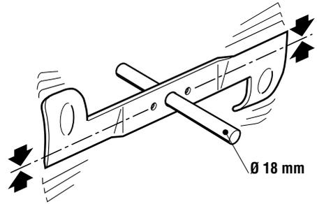
**⚠ WARNING!** Damaged or bent blades must always be replaced; never try to repair them! ALWAYS USE MANUFACTURER'S GENUINE REPLACEMENT BLADES BEARING THE SYMBOL **▲!**
