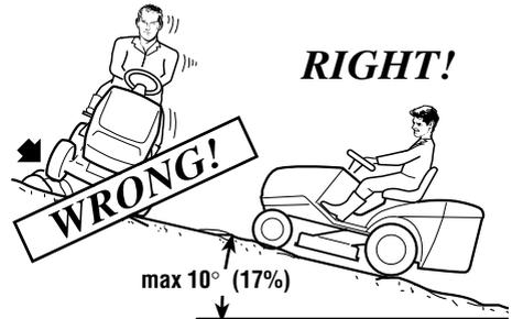
**⚠ DANGER!** **REDUCE SPEED BEFORE ANY CHANGE OF DIRECTION ON SLOPES, and always engage the parking brake before leaving the machine stopped and unattended.**
