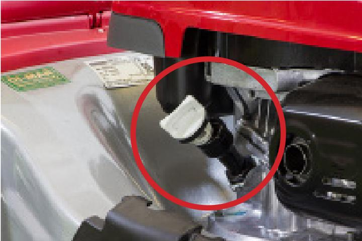
The oil comes out of the lawnmower the same way in which it entered as there is no sump plug on these engines.
