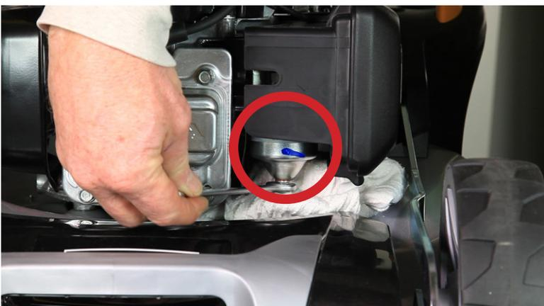
This picture shows a Honda engine from the front of the lawnmower. To the right of the plate with "HONDA" on it, you will see the bottom of the carburetor float bowl. There is a bolt on the bottom of the float bowl. Place a suitable container underneath the float bowl to catch the fuel and using a 10mm spanner loosen the bolt at the bottom of the float bowl. The fuel will drain into the container. Tighten the bolt again after all the fuel has been drained from the lawnmower.
