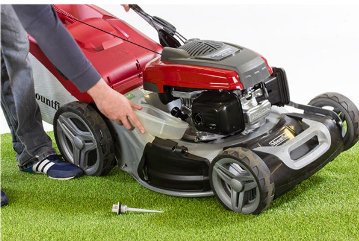
If you do not have an oil syphon or syringe, you can tip the lawnmower sideways to pour the oil out.
