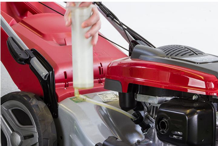
Using a suitable oil syringe or syphon, remove the oil from the engine via the oil fill tube.
